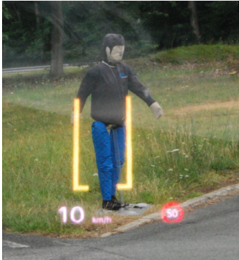
Figure 1: Picture of a real scene with superposed virtual image generated by the AR windshield HUD system
